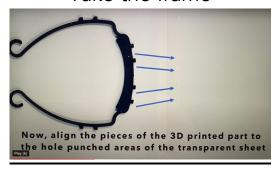
Take the shield and align the holes with the pegs on the frame.
